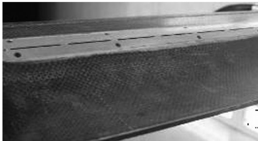
Fig. 9 A rear view of the Glauert section of the wing with the actuator exit slots. Each slot is 40 by 1 mm, with 5 mm of separation between each actuator pair. A 12-actuator array was installed in each wing.
